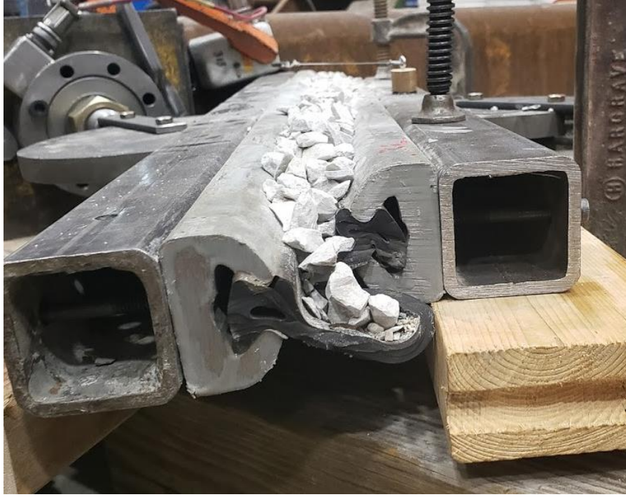
Figure 27: Increased Racking Due to Debris
