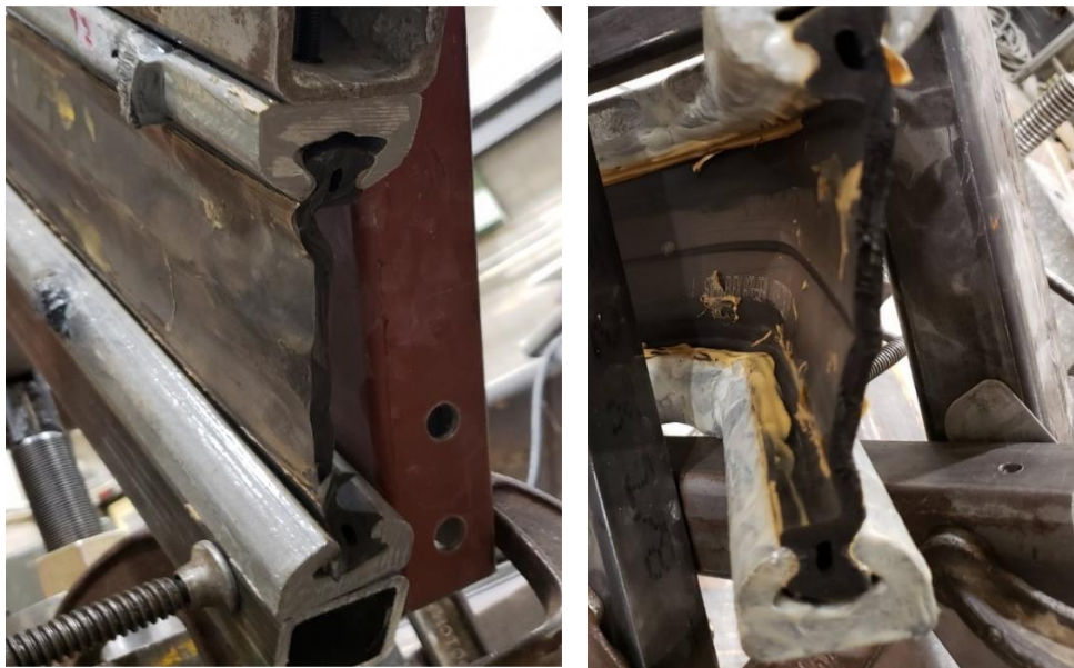
Figure 15: Typical A2R-400 Behavior in Extension
