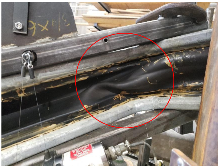
Figure 20: Upturned Section Failing in Closure Following Extension
